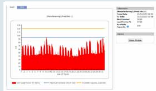
Track consumption profiles of a measuring point over various days of the week
