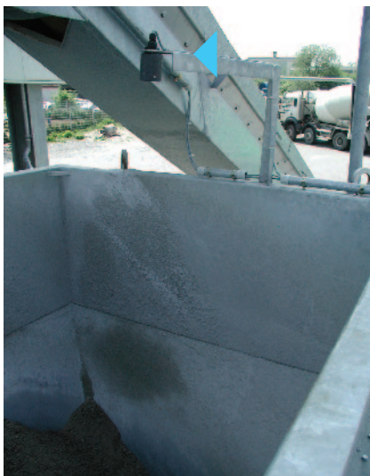
Level measurement in buffer silos for aggregates with Prosonic
