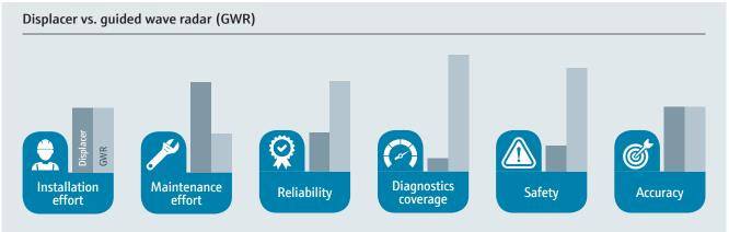
In this distillation application, with volatile surface, a bypass solution is a must for safety. Our customer rated the technical comparison between displacer and guided wave radar as visualized in the graphic.
