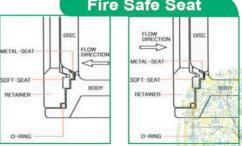
Seat Material Maximum Working Temperature SS316L \* RPTFE 230°C (446 F) FIRE-SAFE to API 607 5th Edition SEAT LEAKAGE-Leakage of soft seated version is Zero
